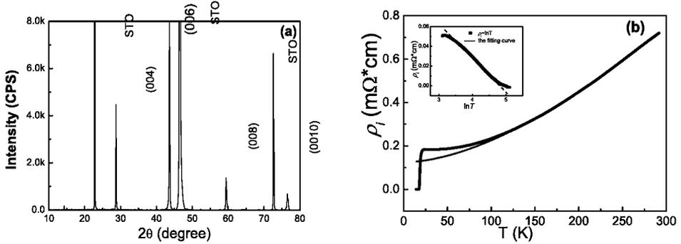
Fig. 1. (a) X-ray diffraction spectra of the LCCO thin film, *c*-axis oriented on the (001) STO substrate. (b) Temperature dependence of resistivity in the thin film with  $x=0.09$ , the dash line is the background,  $\rho_0+\rho_s$ . Inset gives  $\rho_i \sim \ln T$  which is obtained by subtracting  $\rho_0+\rho_s$  from the experimental data, the dash line is from the fit to the Kondo effect (formula (2)) in zero field.
