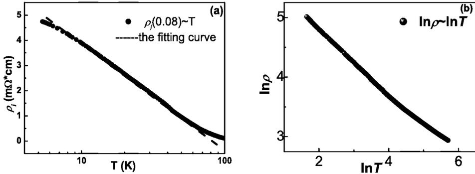
Fig. 2. a)  $\rho_i$  -  $T$  curve of LCCO with  $x=0.08$  is plotted as single logarithmic relation. In the temperature range of 10-70 K, the experimental data and the fitting curve by formula (2) overlap very well. b)  $\ln \rho_{ab} \sim \ln T$  curve, the slope of the linear curve is about 0.5. The physical meaning will be studied further.
