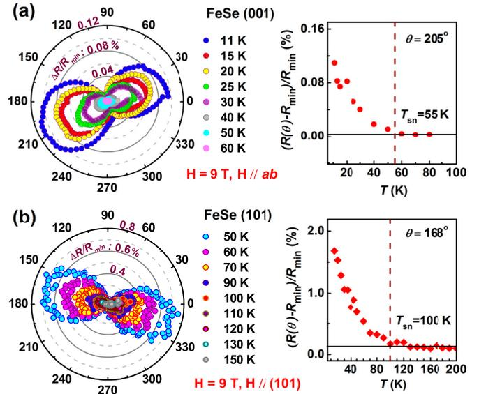
FIG. 2. Temperature dependences of the angular-dependent magnetoresistance showing the twofold rotational symmetry below  $\sim 55$  K (the upper right) and  $\sim 100$  K (the lower right). (a) The FeSe crystal sample of (001) orientation with  $T_c \sim 7.6$  K. (b) the sample of (101) orientation with  $T_c \sim 10.0$  K. The  $\theta$  is the angle between the directions of the external field ( $H$ ) and the current ( $I$ ), with  $\theta = 0^\circ$  corresponding to  $H \perp I$ .
