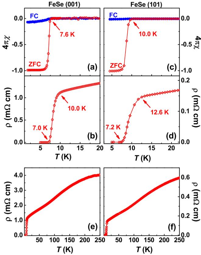
FIG. 1. Temperature dependences of the static magnetic susceptibility, corrected for demagnetization factor, and the electrical resistivity for the two typical FeSe single crystal samples with (001) and (101) orientations. (a) and (c) The data of magnetic susceptibility; (b) and (d) the electrical resistivity near the superconducting transitions; (e) and (f) the resistivity up to 250 K. The magnetic measurements are performed under  $H = 1$  Oe.
