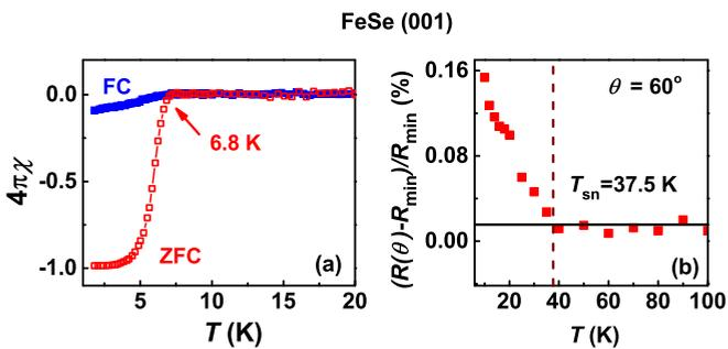
FIG. 3. (a) Temperature dependence of the static magnetic susceptibility for the hydrothermal FeSe crystal sample of (001) orientation with the  $T_c \sim 6.8$  K. (b) Its temperature dependence of the maxima in anisotropic AMR showing the  $T_{sn} \sim 37.5$  K. The  $\theta$  is the angle between the directions of the external field ( $H$ ) and the current ( $I$ ), with  $\theta = 0^\circ$  corresponding to  $H \perp I$ .
